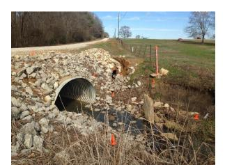
Preliminary trials on structure for motion using soccer cones for reference points. We measure between the cones on the ground and in the image to validate our 3D surface model. We are able to also make some really neat visuals of our work that can be viewed by stakeholders. This link will access one of those videos. <u>https://goo.gl/gWCfmv</u>
