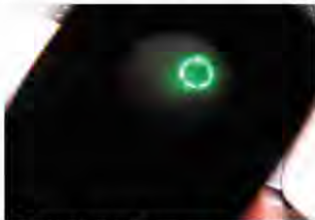
Fig. 7 End view of an FFSC TW under a microscope as a light beam from a green LED guided through the FFSC.
