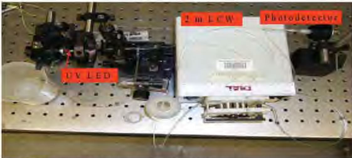
Fig. 2 A photograph of a laboratory set-up of the Cr(VI) sensor.
