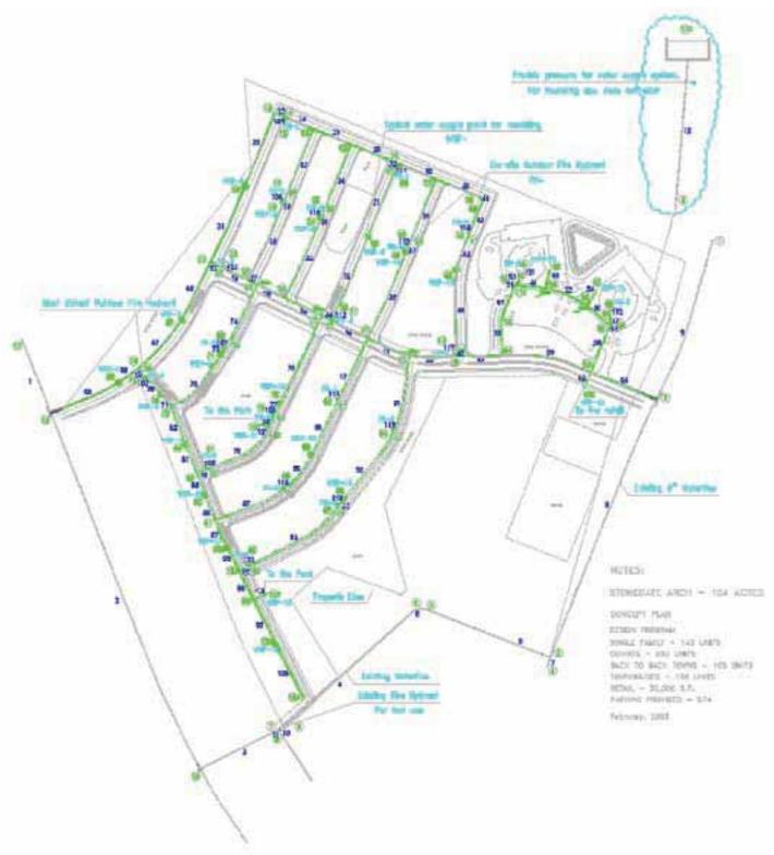
Figure 2. AutoCAD Conceptual Plan of Water Supply System
